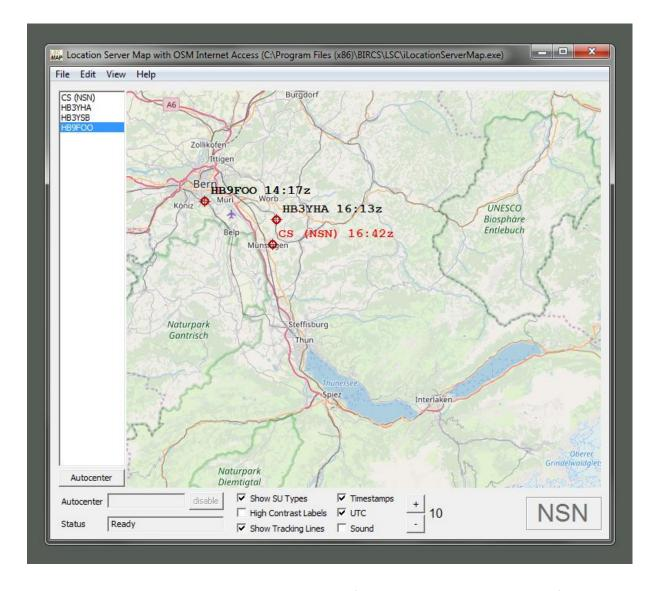
Since LSC logs location data received by the SUs in the field as day logs the map display of any point in time can be traced whenever it is necessary using the program Location Server Map Replay (LSM Replay). Location data is archived for a maximum of one year but can be deleted anytime if desired.
