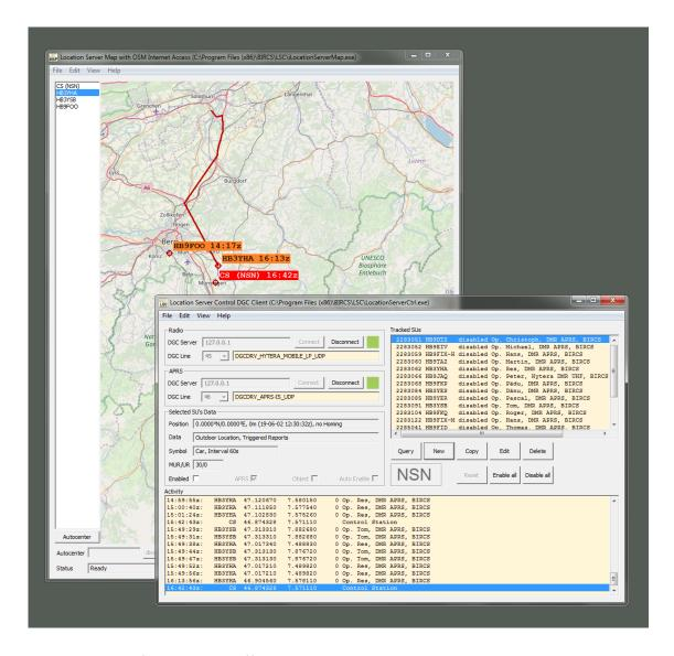
LSC maintains logs of all location traffic. This data can be visualized and replayed anytime during one year from the time it was recorded. Location Server Map (LSM) serves as a real time mapping module working with individual locally stored (offline) raster bitmap maps for displaying the SU's location.
