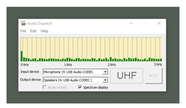
Similar to RRC and RRC/R there is a program variant AD/R intended for direct repeater access. With AD/R audio streams between a dispatcher PC and a repeater are transmitted or received using a LAN/WAN network connection without any radio (available for Hytera systems only).
